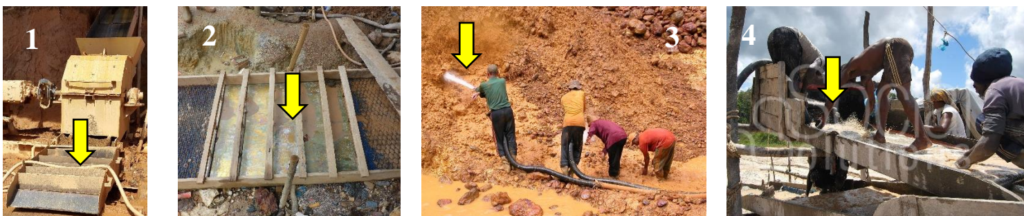
Figure 5. Locations where mercury is usually added; in the "safe" of the hammer mill (1), on the copper plate (2), on the ore while sluicing (3), and/or when washing the sluice box (4). Methods 1-2-3 are examples of Whole Ore Amalgamation.
